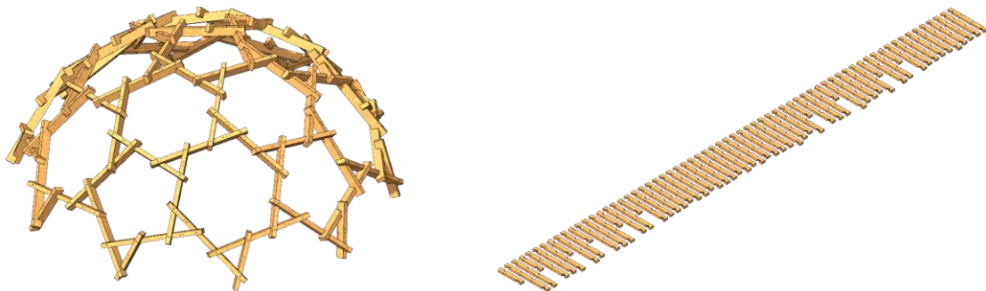
Figure 6.3: Baked RFD model and its unfolded version ready for design to production. Diameter of the full-scale dome is 10 meter
