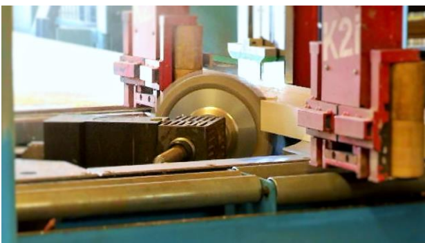
Figure 6.14: Fabrication of the mock-ups with the milling tool of a Hundegger K2i at Heko Spanten
