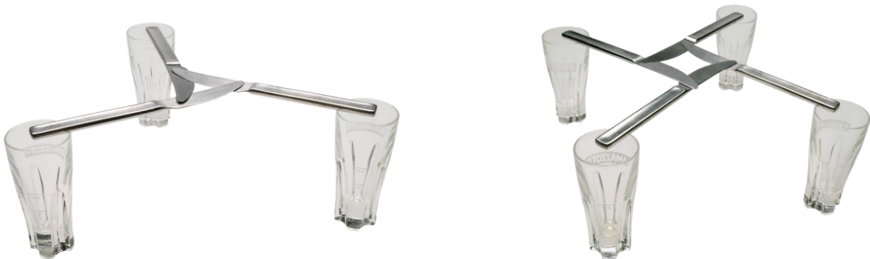
Figure 2.1: The structural principle of a three- and four-member single unit reciprocal frame
