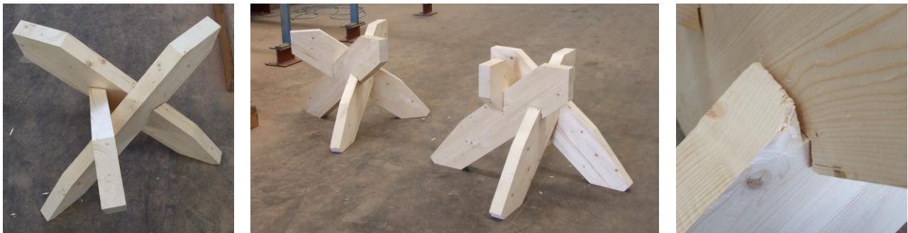
Figure 6.15: Full scale mock-up made with Hundegger K2i at Heko Spanten
